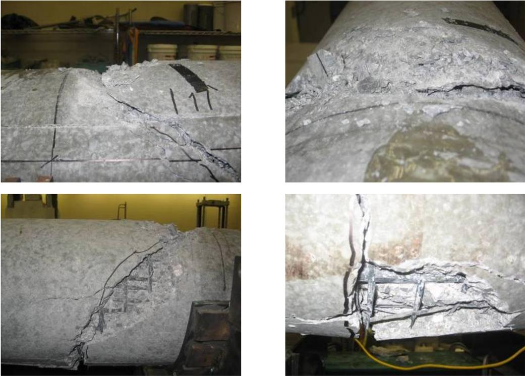
Figure 17: Concrete failure for poles confined with C-GRID
