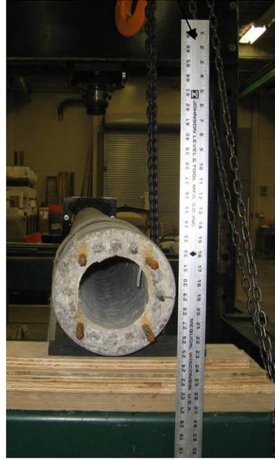
Figure 12: Deflection measurement at pole tip end
