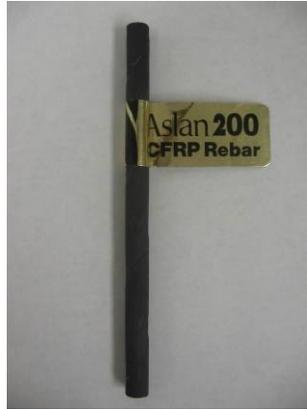
Figure 1: Aslan 200 CFRP rebar sample
