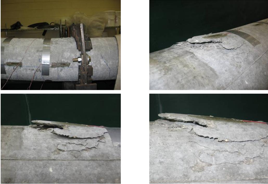
Figure 16: Concrete crushing at failure for poles confined with steel spirals
