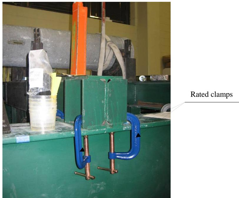
Figure 9: The clamp fixation of the supporting beams
