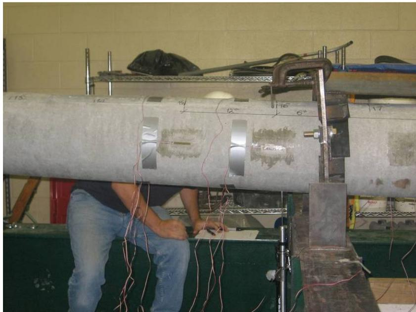
Figure 11: Strain gages location at 6 in and 18 in from the support
