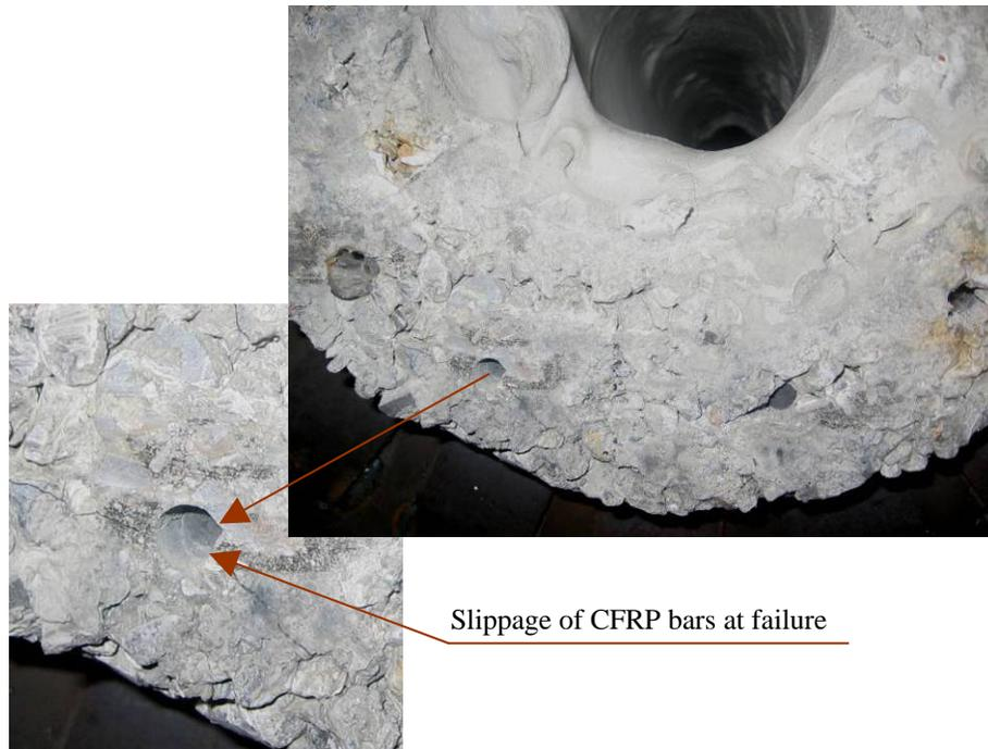
Figure 18: Slippage of CFRP bars at failure of poles confined with C-GRID
