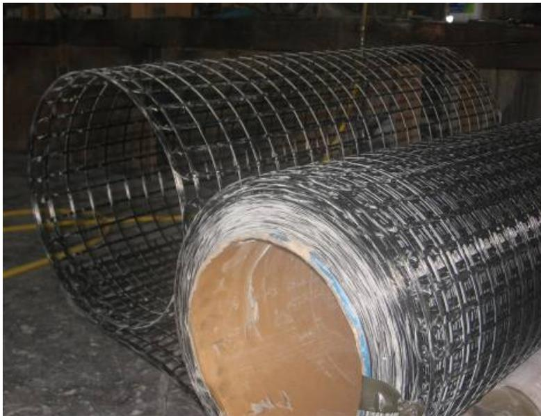
Figure 2: C-GRID CFRP grid sample
