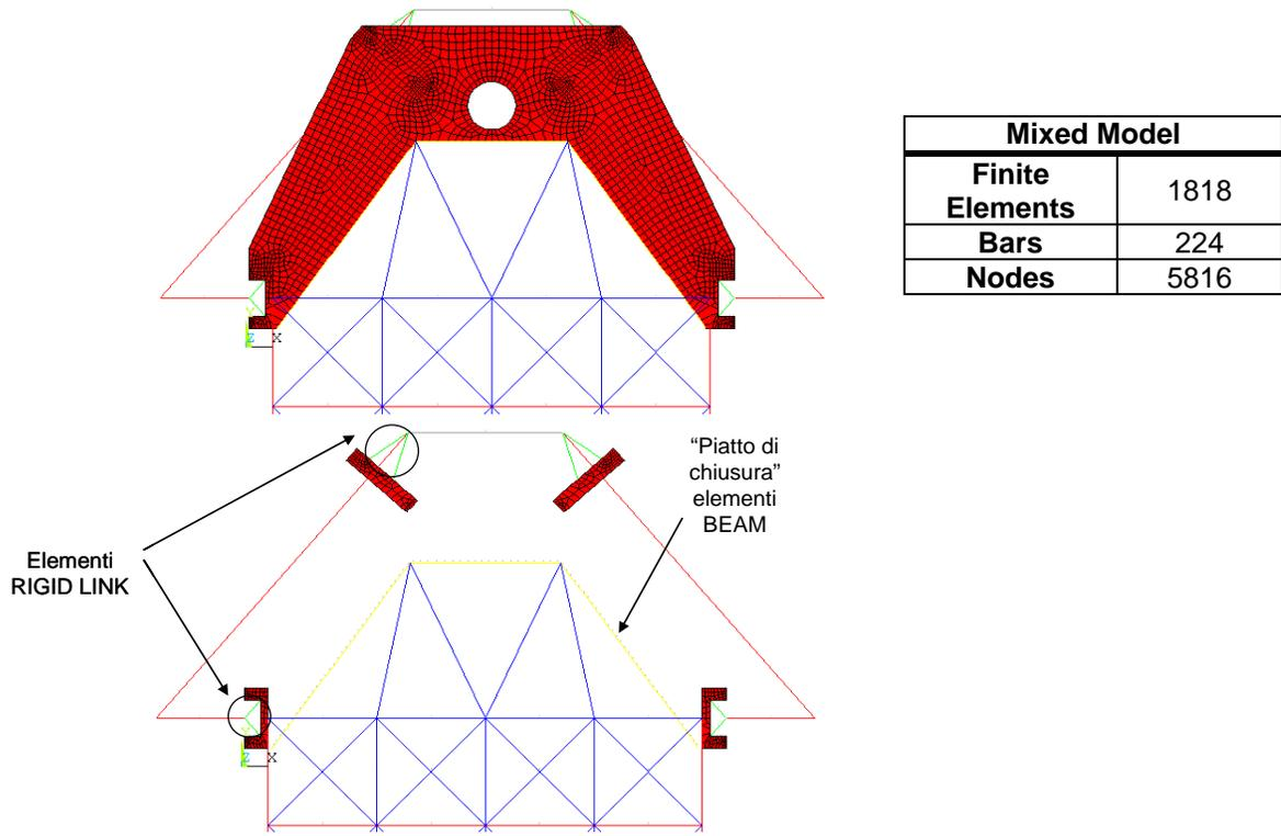
Fig.9: Mixed model: top, main frame, bottom, details for the restraints of the stays.
