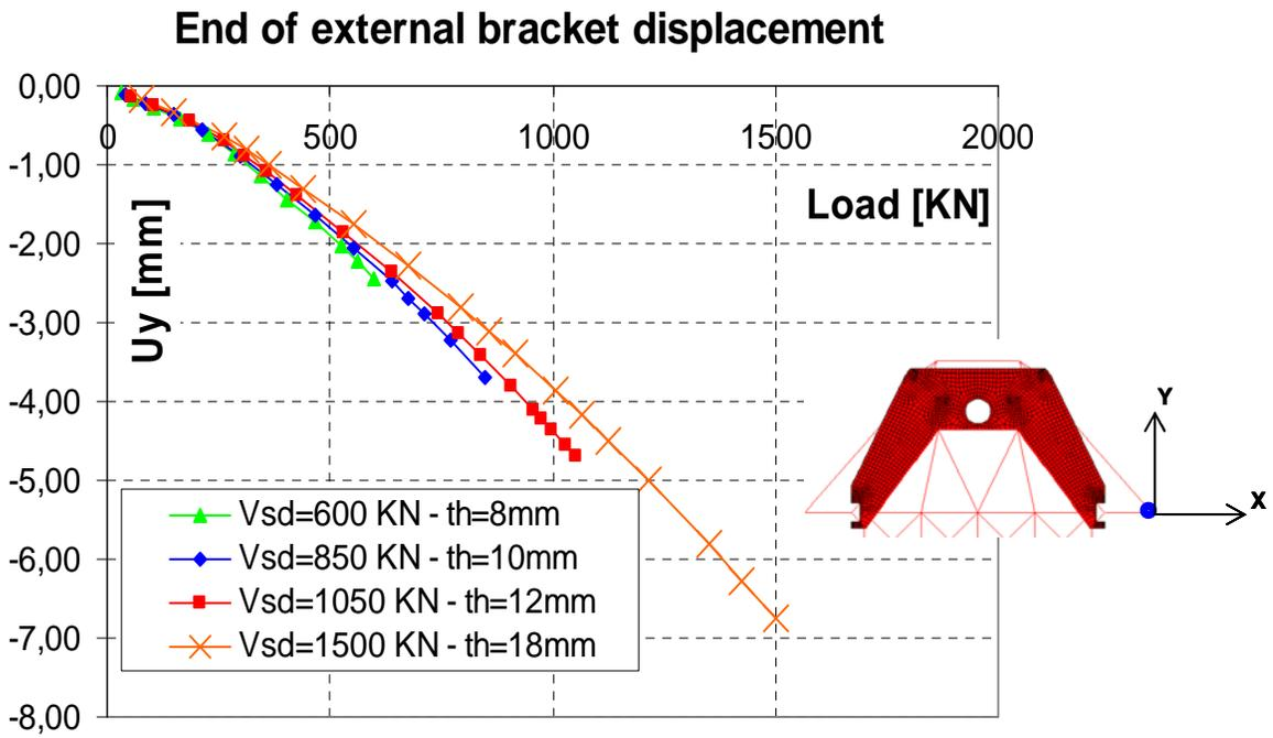
Fig.11: Load-displacement for the external point of the bracket, for the symmetric cases.
