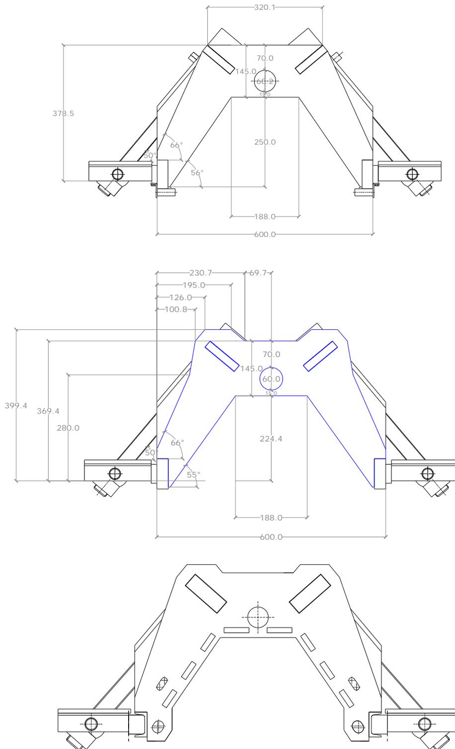
Fig.14: Evolution of the configuration of the cable-stayed bracket as consequences of the development of the analysis.
