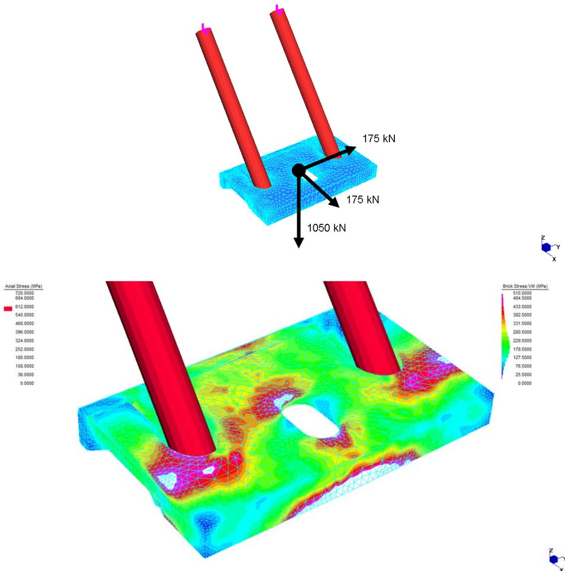
Fig.19: Typical load configuration considered and stress state contour obtained during the optimization process of the external bracket.
