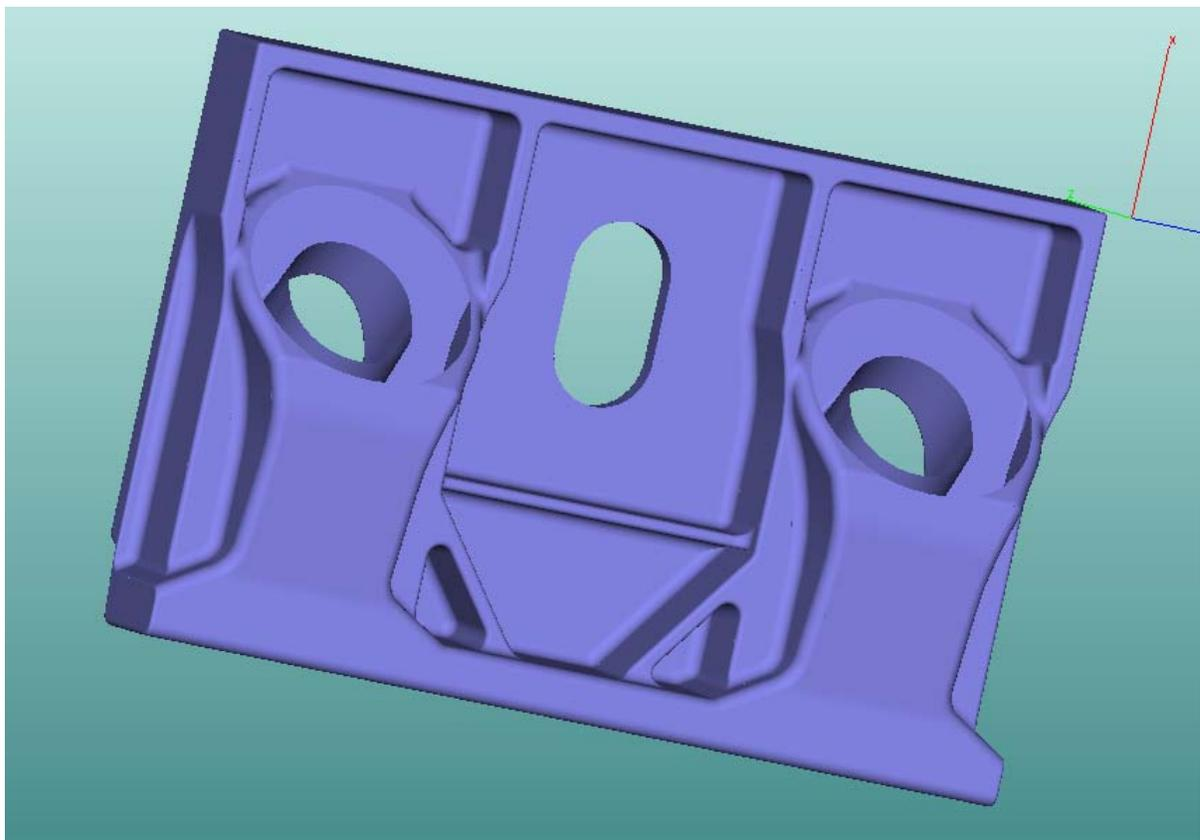
Fig.20: Top and bottom view of the finally obtained configuration of the external bracket.
