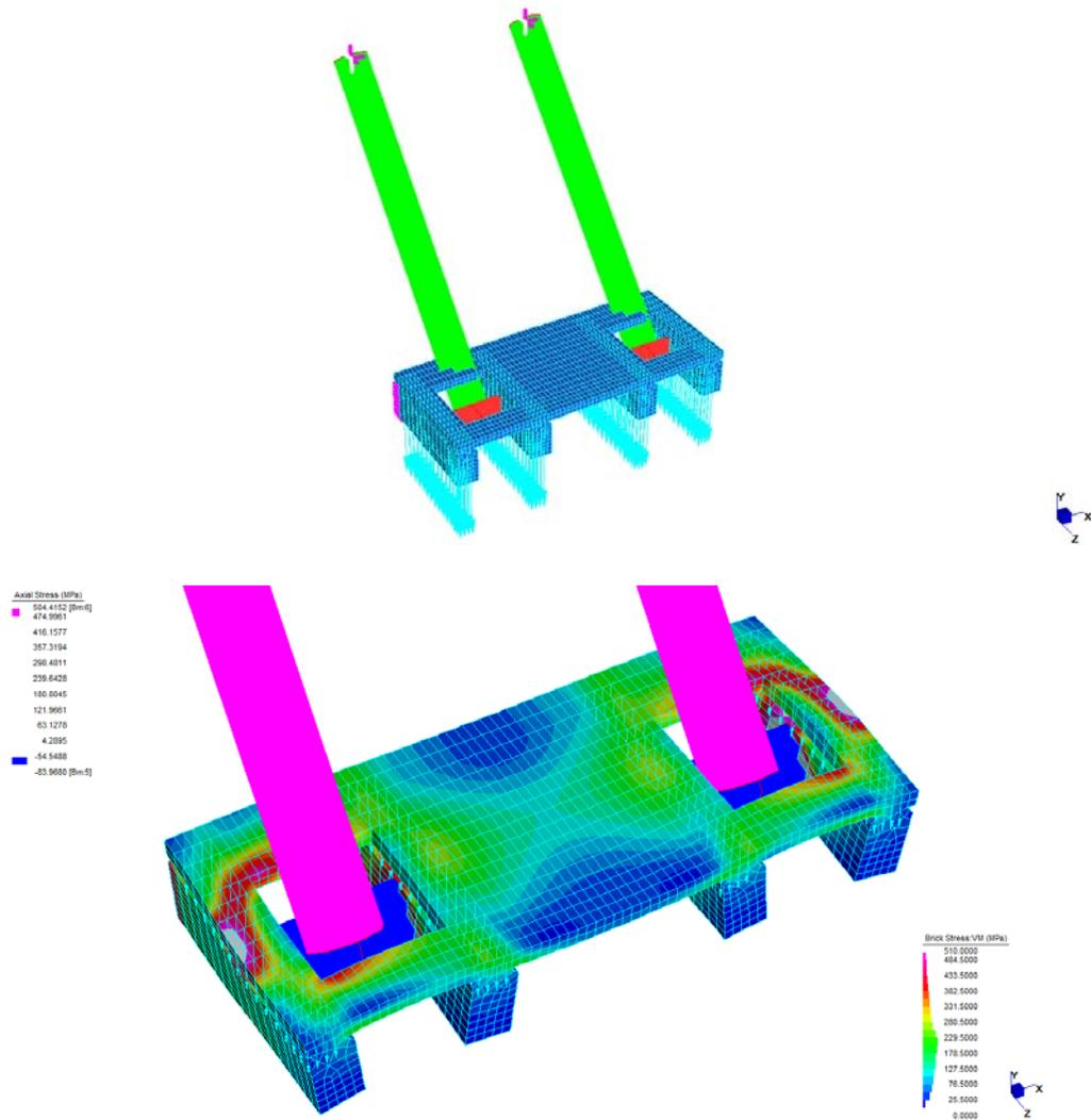
Fig.17: Initial configuration of the external part of the cable-stayed connection and, on the bottom, typical stress state after load application.
