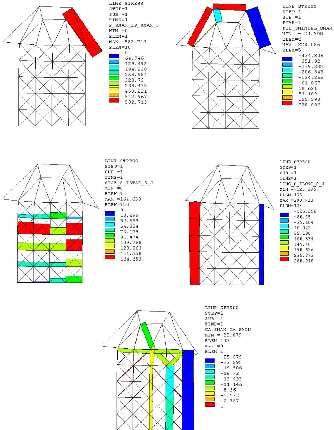
Fig.8: Typical results from S&T model: for the asymmetric load, on the top, axial actions on the bars representing the frame of the connection, in the middle stress on the stirrups and on the longitudinal bars, on the bottom, stress on the concrete core (please note the no tension response).
