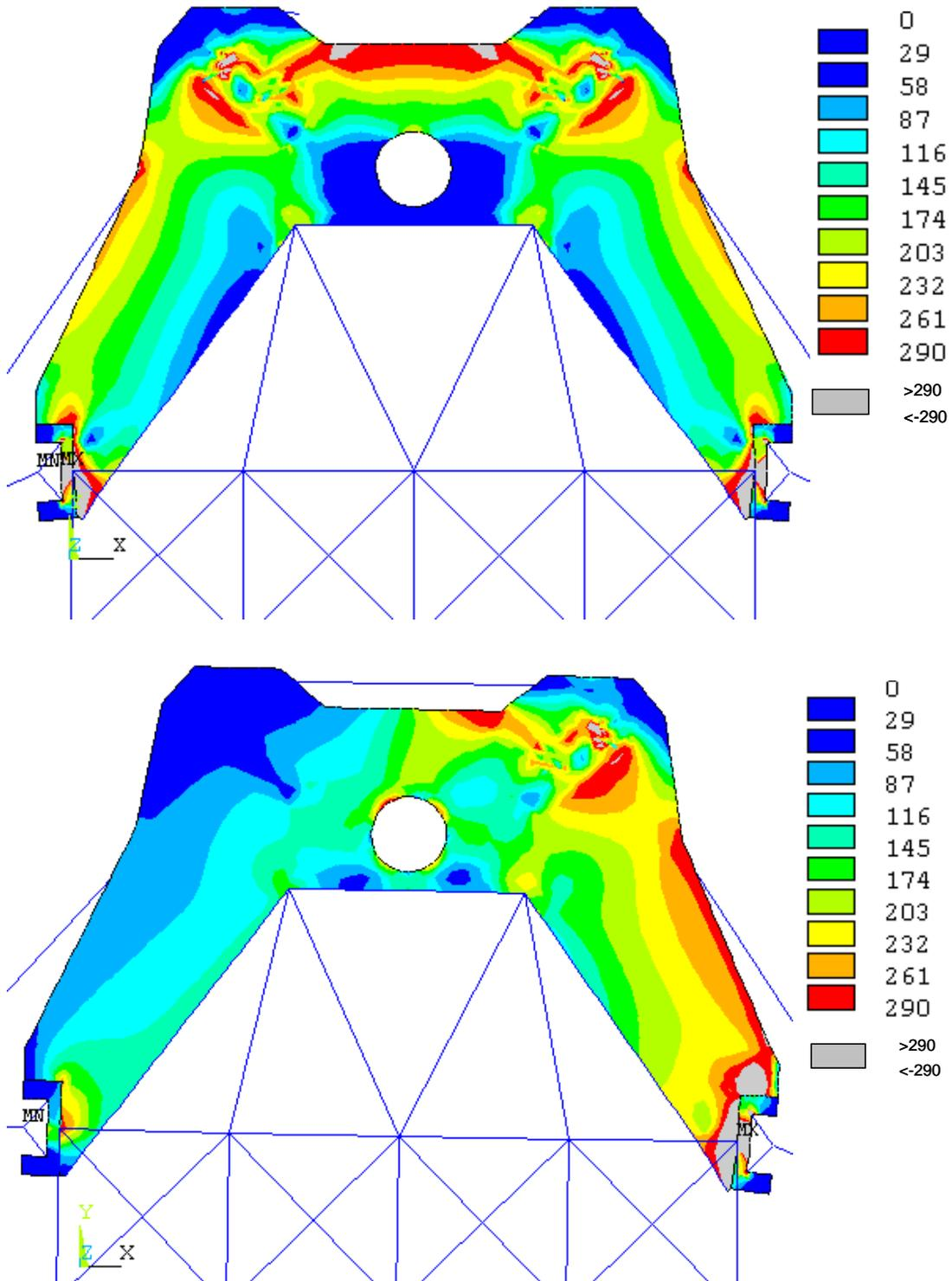
Fig.13: Stress field for the Von Mises Yielding Criteria for  $V_{sd} = 1050$  KN, adopting for the frame plates a 12 mm thickness: on the top, symmetric case, on the bottom, asymmetric case; in gray are enlightened the regions where yield is reached.
