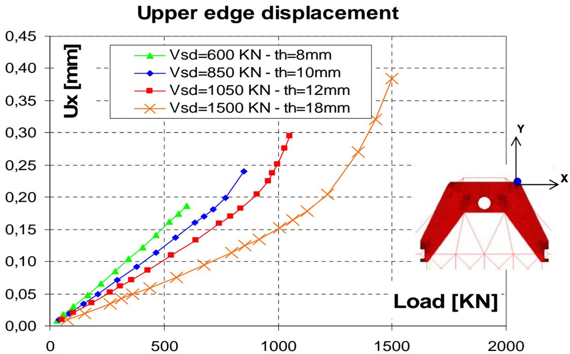
Fig.12: Load-displacement for the external point of the frame, for the symmetric cases.
