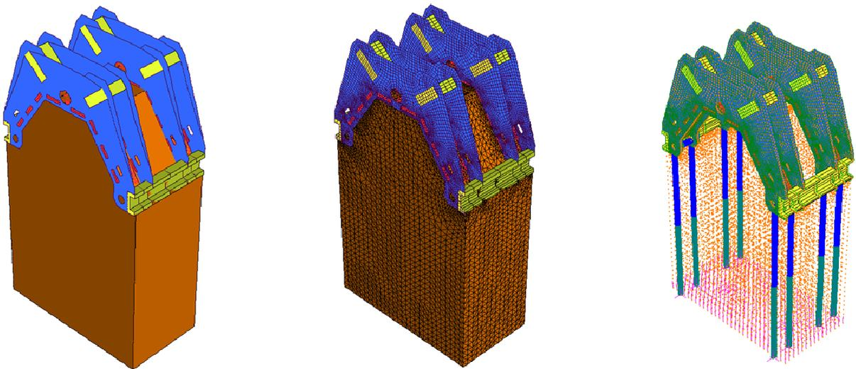
Fig.15: Three-dimensional modeling of the connection and of the segment of concrete columns; on the left, only the steel parts (plates of the frame and longitudinal bars) are represented.
