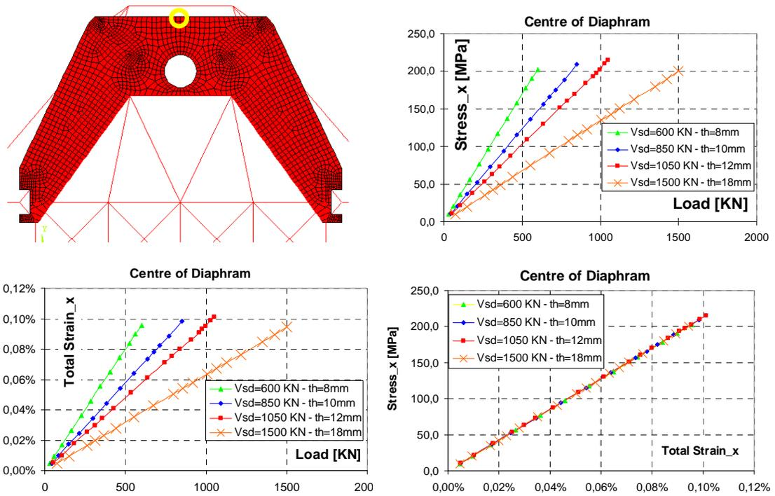
Fig.10: Load-stress and load strain diagrams under symmetric loading case (marked point).
