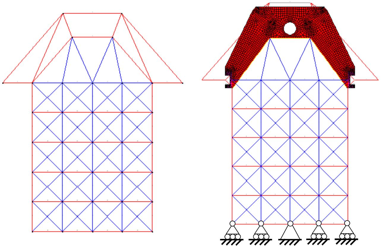
Fig.6: Full discrete (S&T) and mixed (FEM – S&T) modeling of the connection with base restraints.
