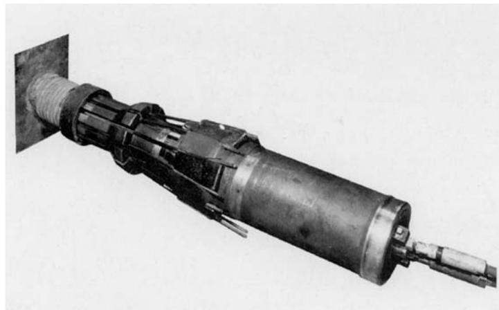
Figure 7 - Concrete anchorage cone and tensing jack
