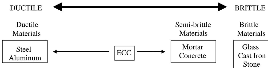
Fig. 1 Range of Ductile to Brittle Behavior of Materials
