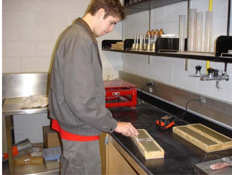
Fig. 4 Casting ECC Bar Specimens
