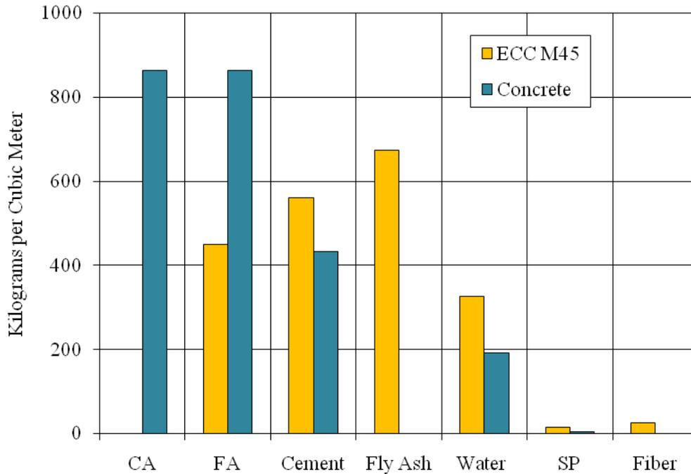
Fig. 3 ECC M45 Mix vs. Typical Concrete Mix
