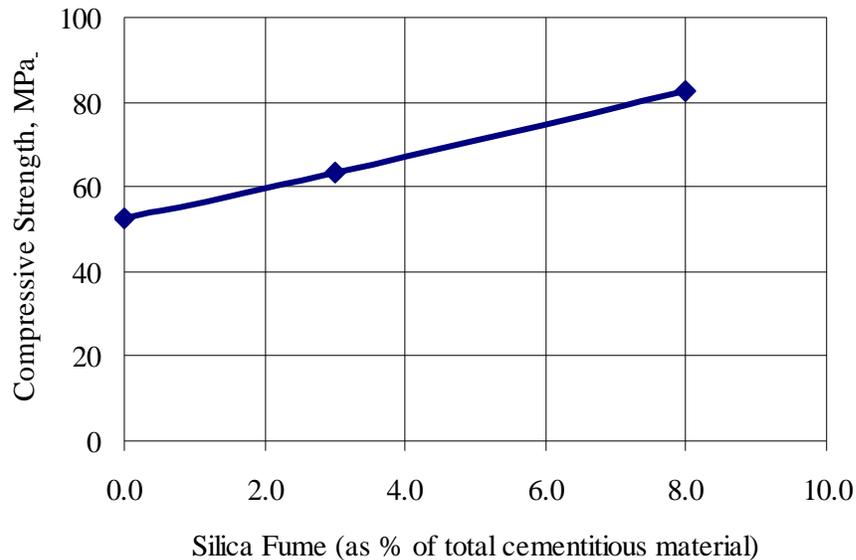
Fig. 9 Silica Fume Effect on ECC Strength
