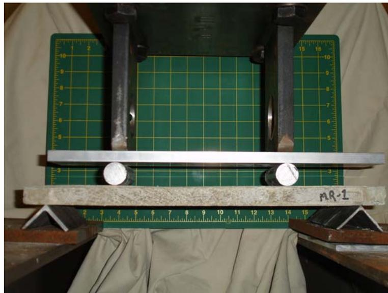
Fig. 5 Four Point Bend Test
