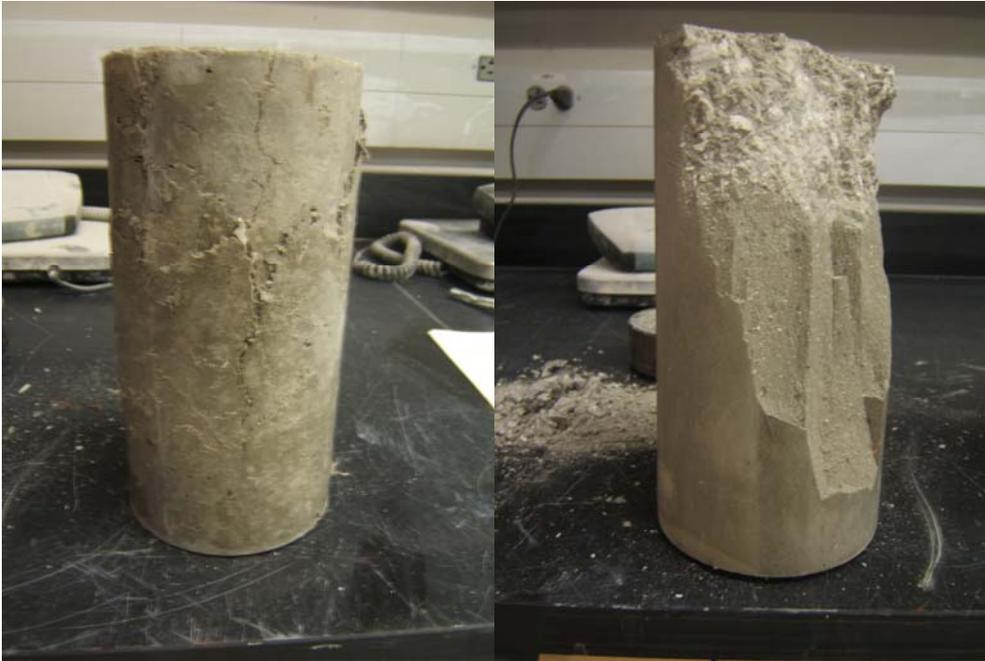
Fig. 11 Compression Test Failures with (Left) and without Fibers (Right) (0.27 w/cm Ratio)
