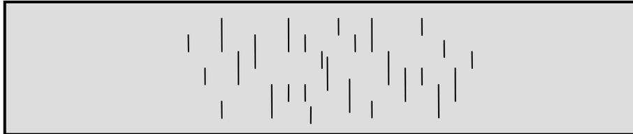
(b) Nonlocalized Cracking of ECC Bars
