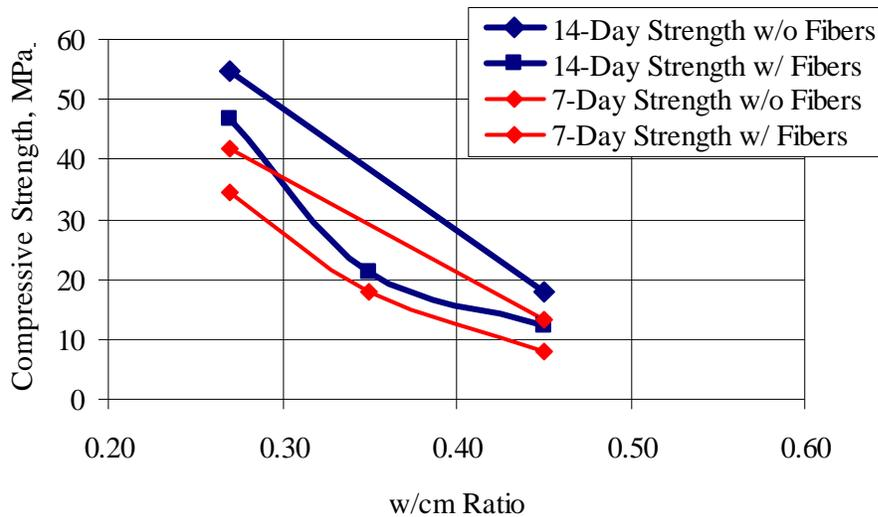
Fig. 10 7- and 14-day Compressive Strength versus w/cm Ratio
