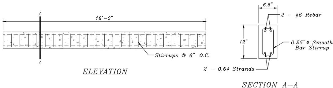
Fig. 1 Typical Beam Specimen Detail
